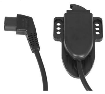
Part No. 81333 Connector **C8** EAN **4251269332** type connector, 999 angled Package Rated current 2,5 A quantity Protection II (Protective Length 85,2 mm class insulation) Height 24 mm Colour black Width 63,2 mm
